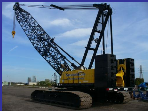
Kobelco CK2000 200 Ton Crawler Crane
